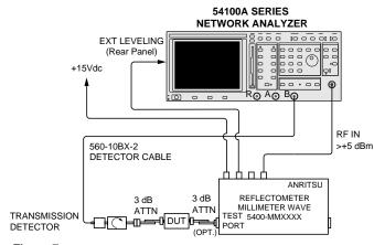
Figure 7 Setup for leveling the output from the 54100A
